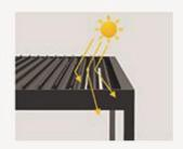
0-120° blade opening and closing angle Refractive dimming
